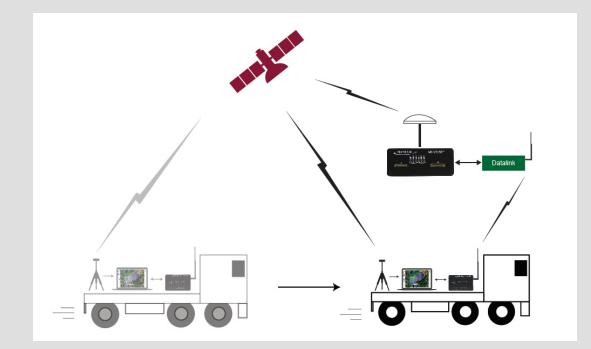
**Location Accuracy** Regular GNSS Dual Frequency RTK Position Accuracy Velocity Accuracy Velocity Accuracy 2.5 m 10 cm
